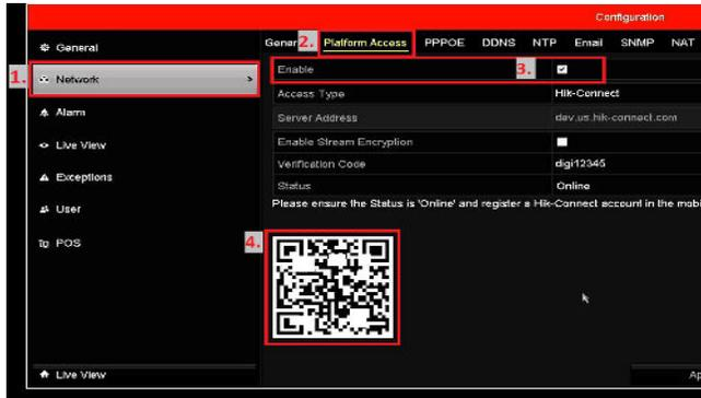
**Step 10:** Right click on NVR > Menu > Configuration > Network > Platform Access > tick "Enable" for Hik-Connect, tick the box, click OK > Apply. Scan the QR code shown on the monitor
