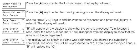
To exit the bypassing mode and return to the Ready state, press the [#] key.
