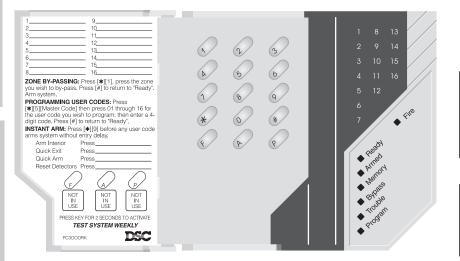
When ON in the normal operating mode, the **Zone Lights** indicate an open zone. eg. open door, window, etc. Refer to zone chart on keypad door for zone information.
